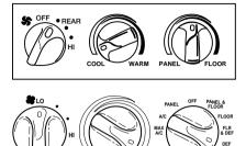
When the auxiliary A/C-heater control is set to FLOOR, airflow only occurs from the third row seat floor vent located in the driver's side rear quarter trim panel.
